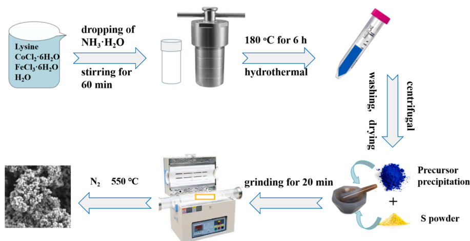
Scheme 1. The preparing procedure of the \text{Fe}_x\text{Co}_{1-x}\text{S}_2 nanoparticles.
