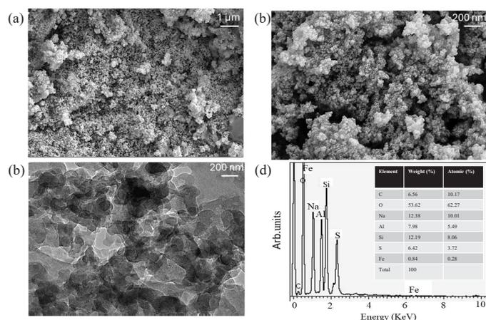
**Figure 2.** Characterization of Si-Al-Fe. (a) Field emission scanning electron microscopy (FESEM) image of Si-Al-Fe with the scale at 1  $\mu\text{m}$ . (b) Field emission transmission electron microscopy (FETEM) with 200 nm scale. (c) FETEM with 200 nm scale. Nanomaterials are uniformly distributed and sized within the range of 20-30 nm. (d) Energy-dispersive X-ray (EDX) of Si-Al-Fe. EDX result confirms the presence of the major elements of Si, Al, Fe, and O in the synthesized material.
