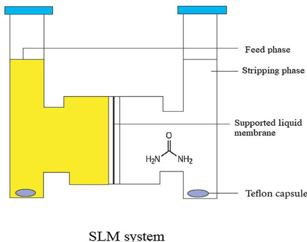
**Fig. 2** Supported liquid membrane (SLM) system for the transport of urea.
