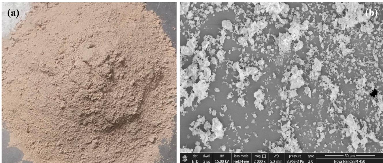
Fig. 1. Waste slate particles (a) Camera image and (b) Microscopic image.
