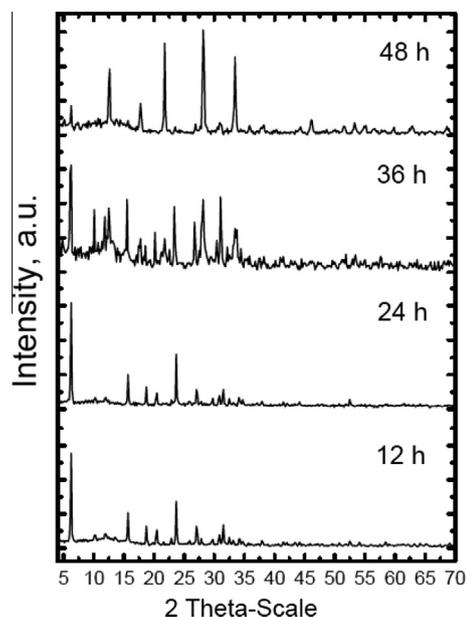
**Figure 6** XRD pattern for two-step synthesis crystallized at different crystallization times.
