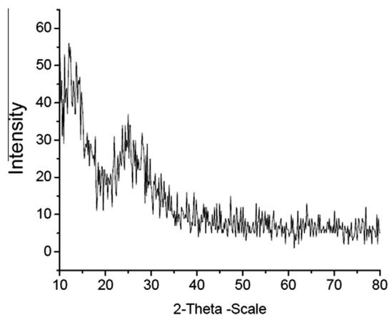
**Figure 3** XRD pattern of silica from RHS.
