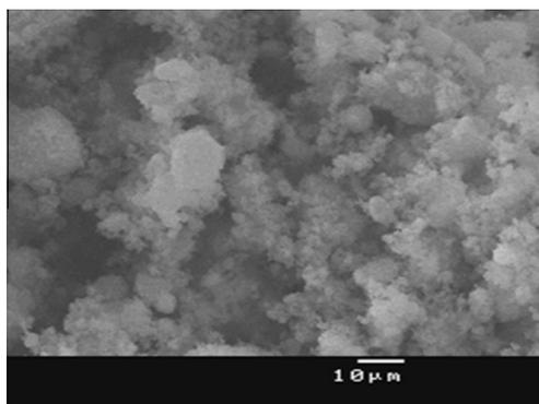
**Figure 4** SEM image for silica from RHS.
