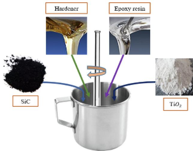
Fig. 2 Preparation of coating solution.
