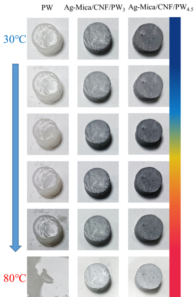
Fig. 6. Digital images of CPCMs thermal leakage experiments.
