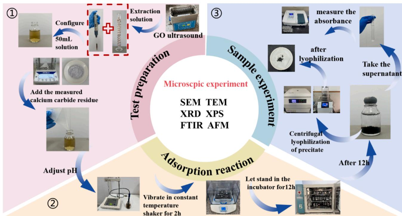
Fig. 1. Flow of adsorption test.
