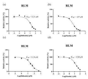
**Figure 6.** IC50 curves of dapsone metabolism in (a and b) RLM and (c and d) HLM by shikonin and fisetin. HLM: Human liver microsomes, RLM: Rat liver microsomes.
