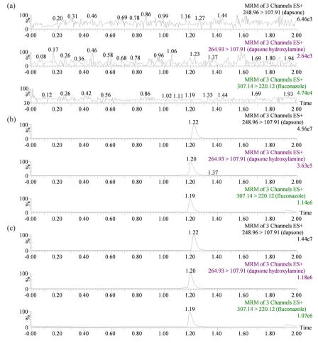
**Figure 2.** Representative chromatograms: (a) Blank plasma free of IS and analytes; (b) The presence of IS and analytes in blank plasma; (c) sample containing IS and analytes after oral administration of 10 mg/kg dapsone from SD rats. SD: Sprague-Dawley.
