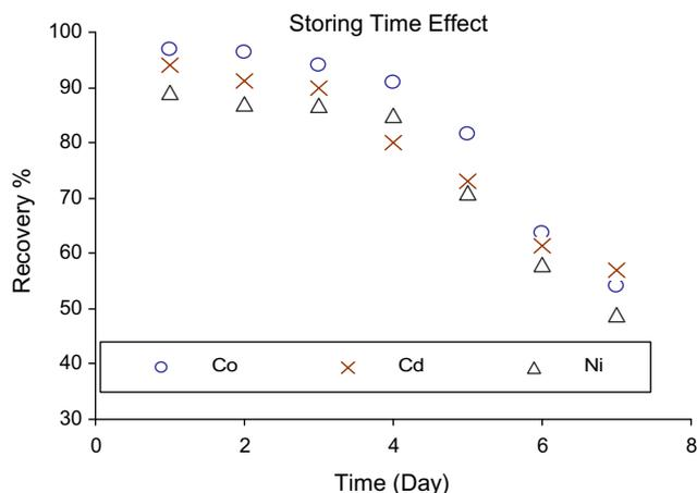
**Figure 8** Effect of storing time on metals recovery.
