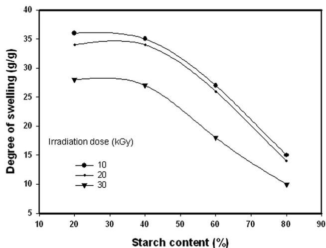
**Figure 4** Effect of starch content on the degree of swelling of Starch/(EG-co-MAA) hydrogels at different irradiation doses and EG:MAA composition; 20:80 wt.%.
