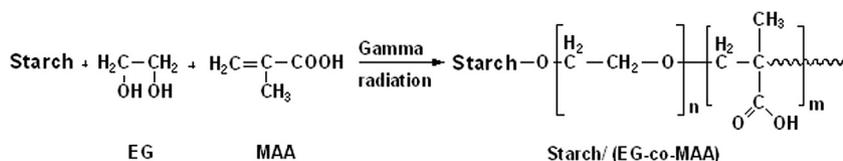
**Scheme 1** Suggested equation for preparation of Starch/(EG-co-MAA) hydrogel.
