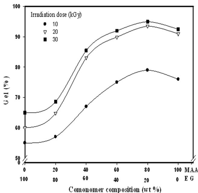
**Figure 3** Effect of EG:MAA composition on the gel (%) of Starch/(EG-co-MAA) hydrogels at different irradiation doses and starch concentration; 40 wt.%.
