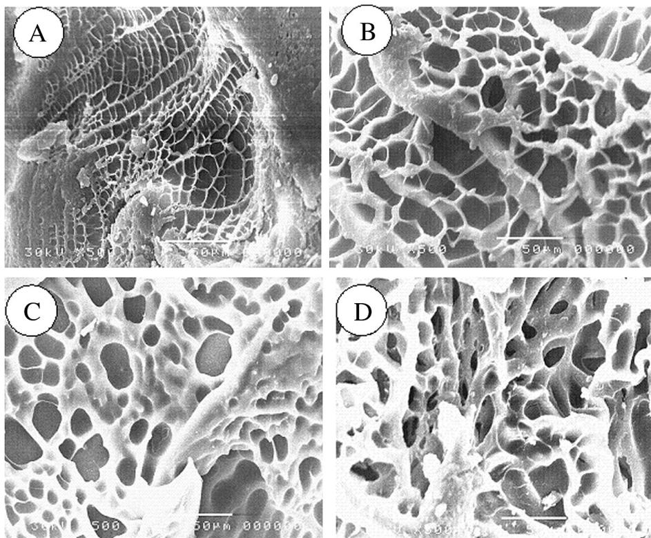
**Figure 7** Scanning electron microscopy of (A) Starch/EG, (B) Starch/(EG-co-MAA) (EG:MAA; 80:20 wt.%), (C) Starch/(EG-co-MAA) (EG:MAA; 60:40 wt.%) and (D) Starch/(EG-co-MAA) (EG:MAA; 20:80 wt.%).
