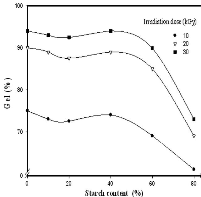
**Figure 2** Effect of starch content on the gel (%) of Starch/(EG-co-MAA) hydrogels at different irradiation doses and EG:MAA composition; 50:50 wt.%.
