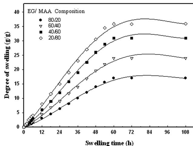
**Figure 6** Swelling rate of Starch/(EG-co-MAA) hydrogels at different EG:MAA compositions. Irradiation dose; 20 kGy and starch concentration; 40 wt.%.
