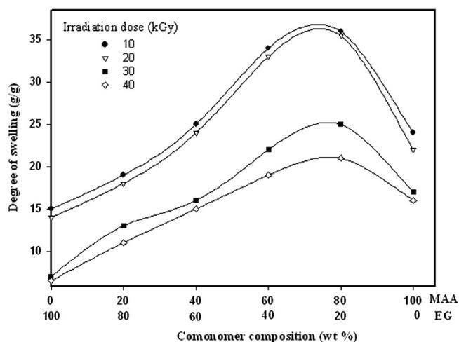
**Figure 5** Effect of EG:MAA composition on the degree of swelling of Starch/(EG-co-MAA) hydrogels at different irradiation doses and starch concentration; 40 wt.%.
