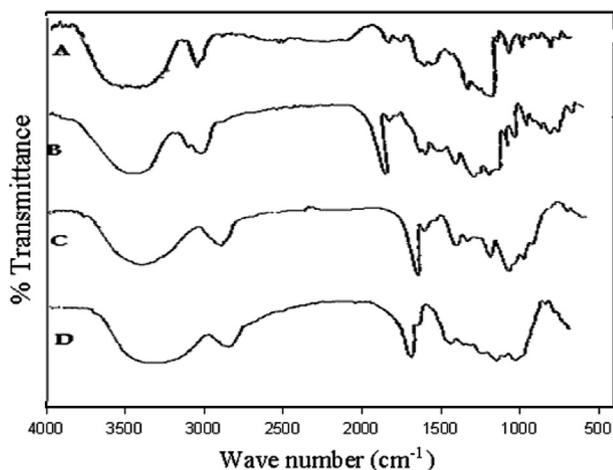
**Figure 1** FTIR of (A) Starch, (B) Ethylene glycol, (C) Methacrylic acid and (D) Starch/(EG-co-MAA) hydrogel.
