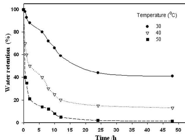
**Figure 11** Effect of temperature on the water retention of Starch/(EG-co-MAA) hydrogels at EG:MAA composition; 20:80 wt.%, irradiation dose; 20 kGy and starch concentration; 40 wt.%.
