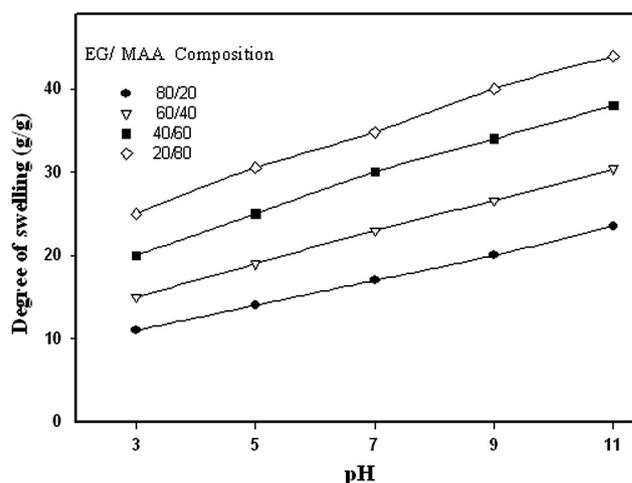
**Figure 8** Effect of pH on the degree of swelling of Starch/(EG-co-MAA) hydrogels at different EG:MAA compositions. Irradiation dose; 20 kGy and starch concentration; 40 wt.%.
