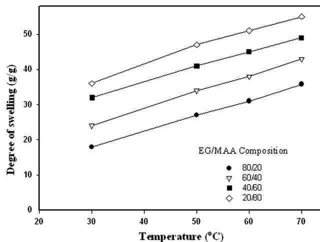
**Figure 9** Effect of temperature on the degree of swelling of Starch/(EG-co-MAA) hydrogels at different EG:MAA compositions. Irradiation dose; 20 kGy and starch concentration; 40 wt.%.
