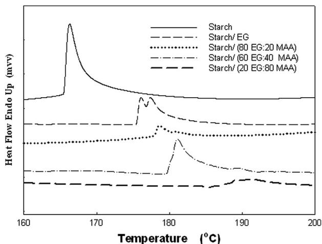
**Figure 12** Differential scanning calorimeter (DSC) diagram of starch and different EG:MAA compositions of Starch/(EG-co-MAA) hydrogels at starch conc.; 40 wt.% and irradiation dose; 20 kGy.
