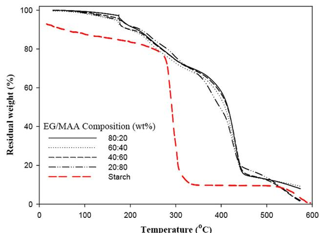
**Figure 13** TGA diagram of starch and different EG:MAA compositions of Starch/(EG-co-MAA) hydrogels at starch conc.; 40 wt.% and irradiation dose; 20 kGy.
