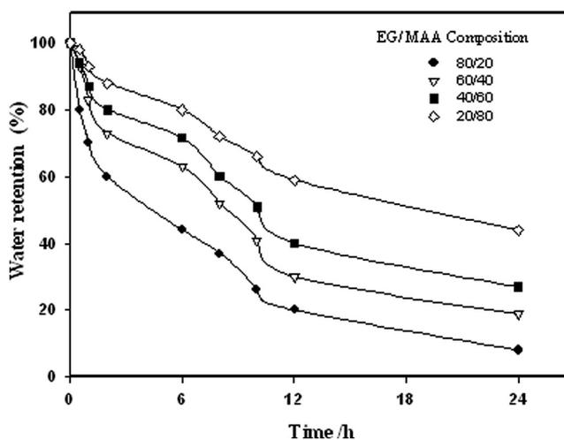
**Figure 10** Water retention of Starch/(EG-co-MAA) hydrogels at different EG:MAA compositions. Irradiation dose; 20 kGy and starch concentration; 40 wt.%.
