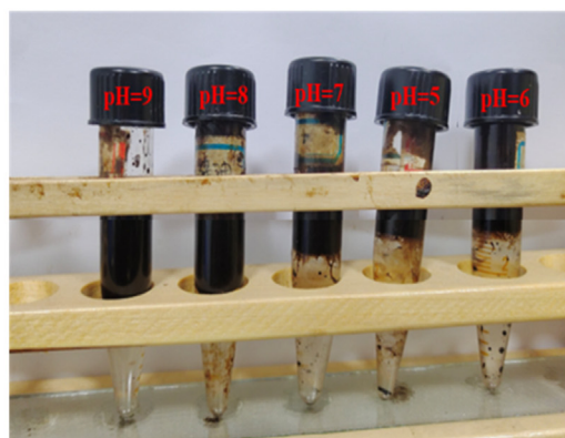
Fig. 7 (a) The demulsification effect of demulsifier at different pH values, (b) Physical diagram of demulsification effect under different pH values in 120 min.
