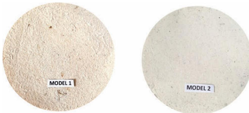
**Fig. 10** The whiteness of pulp without and with bio-catalyst.
