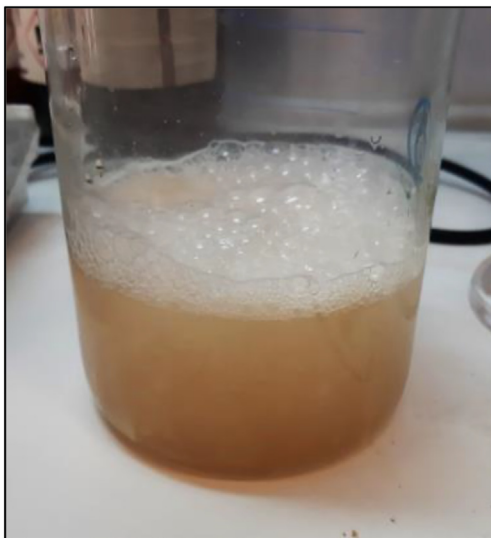
Fig. 26 Mud cake dissolves rapidly in 25% hydrochloric acid.
