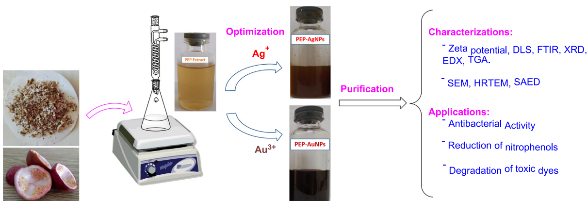
Fig. 1 Schematic illustration for synthesis and application of PEP-AgNPs and PEP-AuNPs biosynthesized by aqueous extract of waste Passiflora edulis fruit peel.
