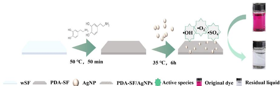
Fig. 1 Preparation process of PDA-SF/AgNPs.
