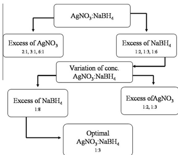
**Scheme 1** Schematic for the preparation of silver NPs.
