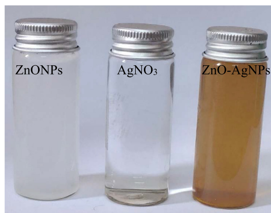
Scheme 1 Optical images of ZnO, \text{AgNO}_3 and ZnO-AgNPs at room temperature.
