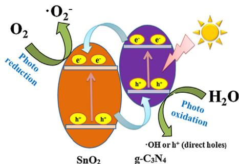
Fig. 12 Schematic illustration of photocatalytic reaction and charge transfer of the S<sub>3</sub> sample under visible-light irradiation.
