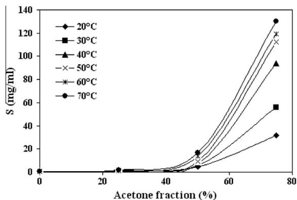
Figure 3 Solubility of AZC as function of water/acetone mixture composition at different temperatures.
