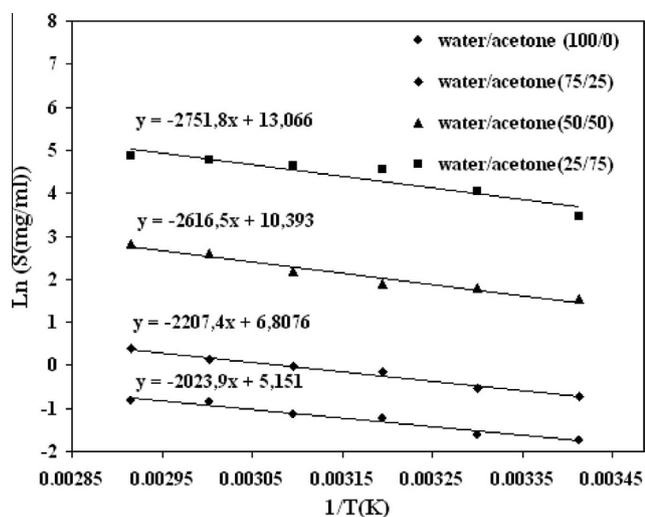
Figure 4 Solubility of AZC as function of temperature for different water/acetone mixtures.
