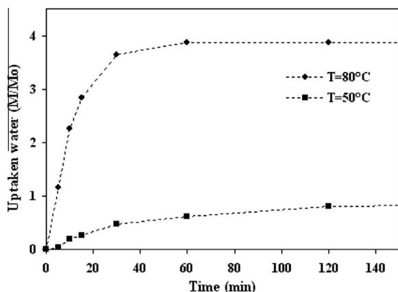
**Figure 6** The rehydration curves of AZ50 and AZ80 in ambient conditions.
