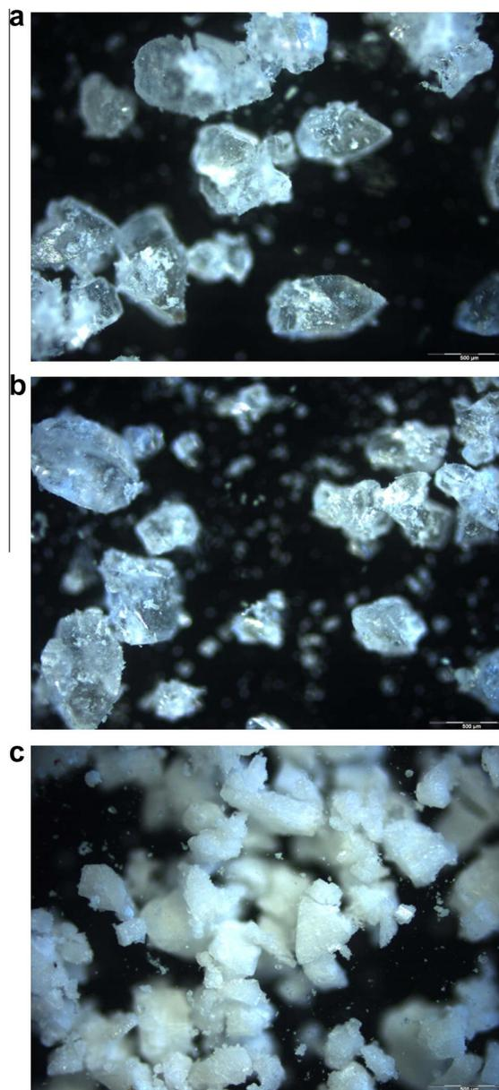
**Figure 1** (a) PLM image of AZC crystals; (b) PLM image of AZ50 crystals and (c) PLM image of AZ80 crystals.
