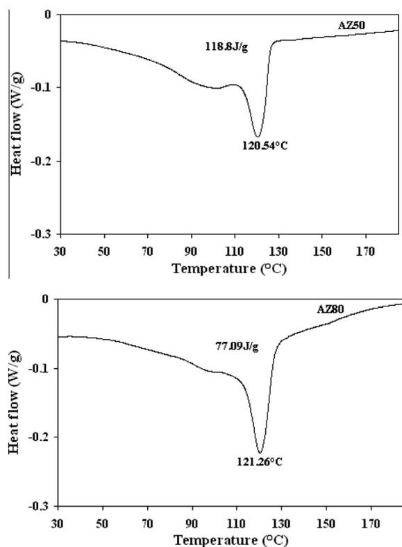
**Figure 8** DSC thermograms of AZ50 (top) and AZ80 (bottom) in open pan.
