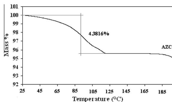
Figure 5 TGA thermogram of AZC.
