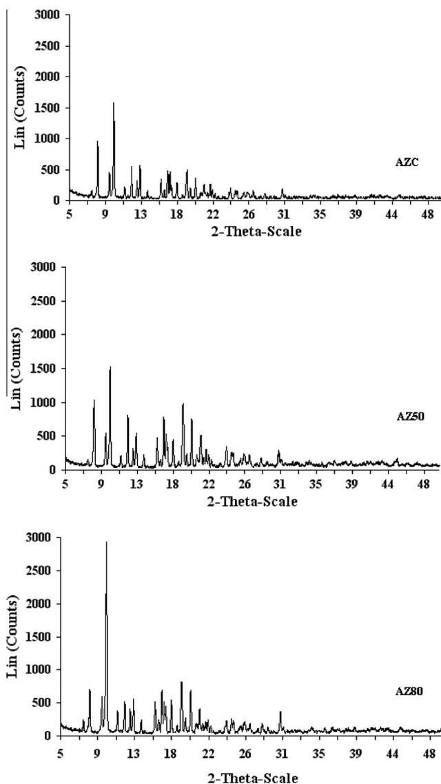
**Figure 9** X-ray diffractograms of AZC, AZ50 and AZ80.
