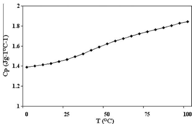
Figure 2 Specific heat capacity of AZC versus temperature.
