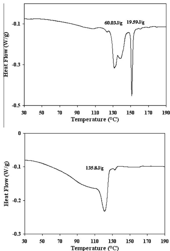
**Figure 7** DSC thermograms of AZC for different pan types: sealed pan (top) and open pan (bottom).
