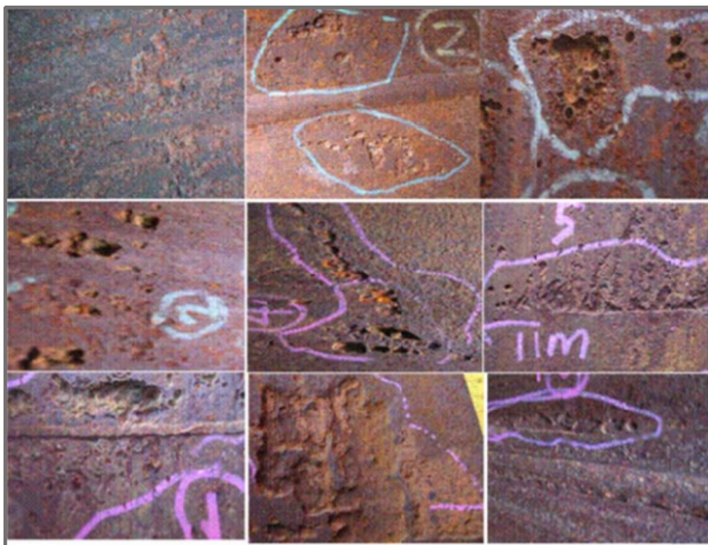
Fig. 10 Typical TLC failure in CO_2 -dominated environments. (Gunaltun et al., 2006).
