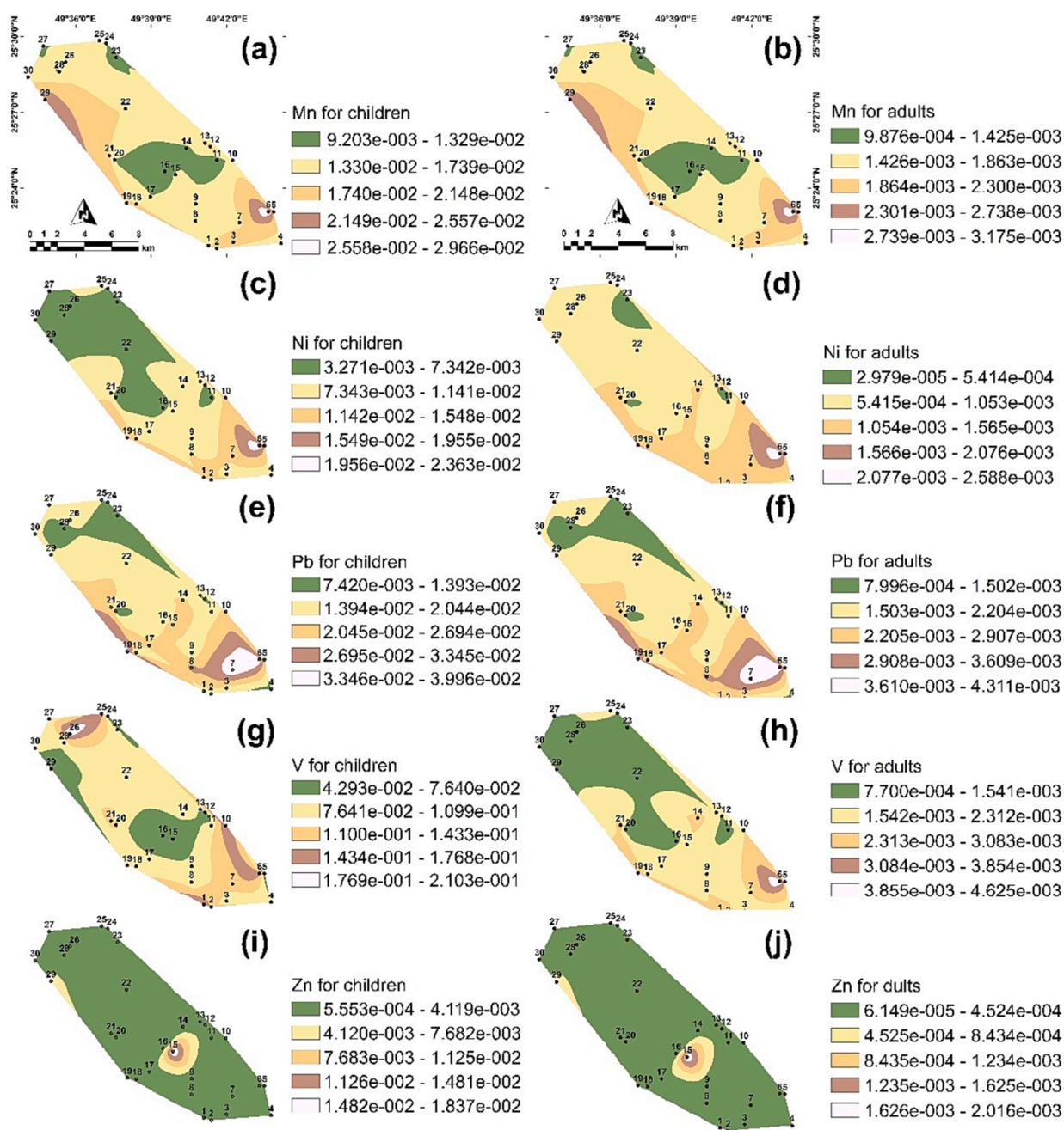
Fig. 5. Spatial distribution of hazard index (HI) of Mn, Ni, Pb, V, and Zn per sampled location.
