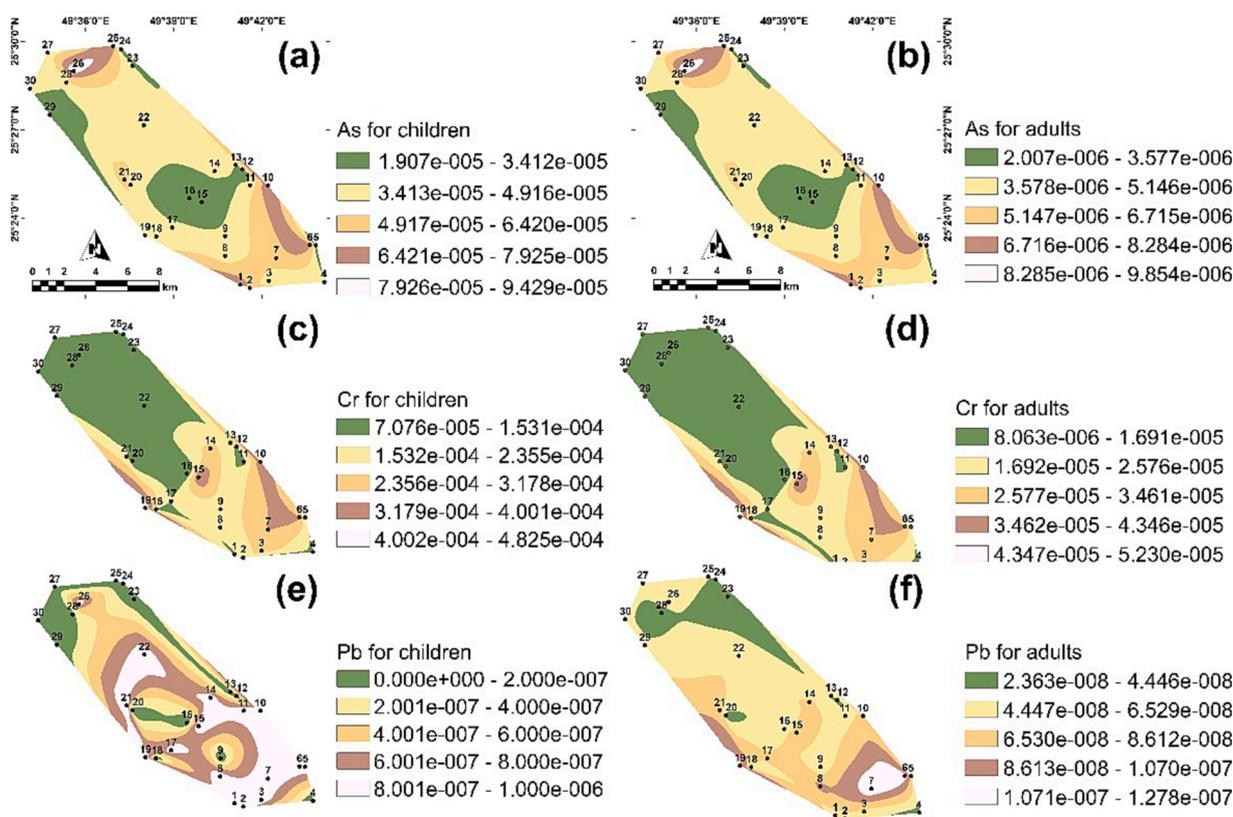
Fig. 8. Spatial distribution of LCR for As, Cr, and Pb per sampled location.
