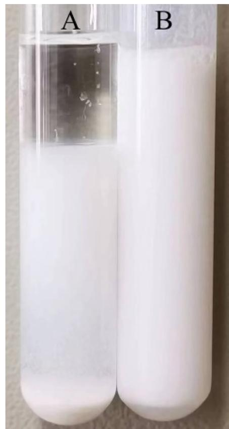
Fig. 1. Digital photographs of the Pickering emulsion stabilized with TiO<sub>2</sub> nanoparticles before (A) and after (B) violent shaking.
