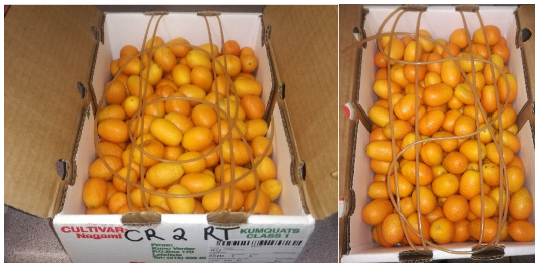
Fig. 1 Photograph of kumquats exposed to the essential oil polymer strands. The strands were impregnated with 20 wt-% of either carvone or spearmint essential oil and 5 wt-% of organoclay Dellite® 43B.
