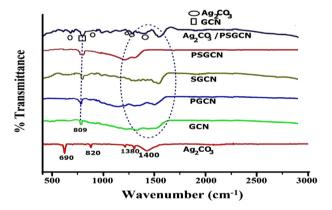
**Fig. 4** FTIR analysis of Ag<sub>2</sub>CO<sub>3</sub>/PSGCN, PSGCN, SGCN, PGCN, GCN and Ag<sub>2</sub>CO<sub>3</sub>.
