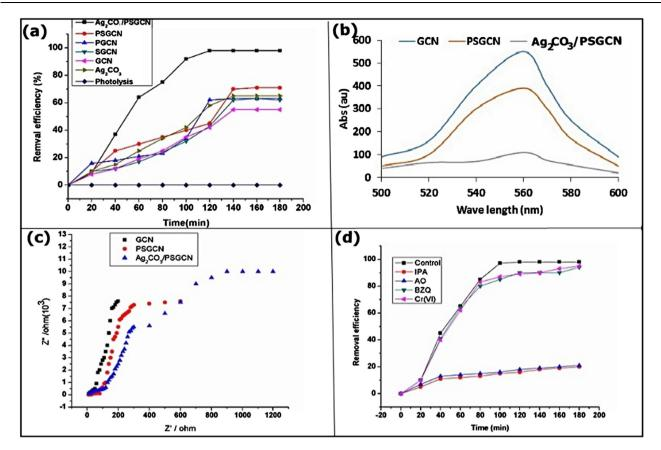
Fig. 8 (a-d): (a) Photo removal of DNP under various reaction conditions, (b) PL spectra of photocatalyst (c) Reaction parameter:  $[DNP] = 1.0 \times 10^{-3} \text{ mol dm}^{-3}$ ; [photocatalyst] = 50 mg/100 mL; initial reaction pH = 4.0 and Light intensity = 750 l×. (d) Effect of scavengers on photodegradation of DNP photocurrent response of photocatalyst.
