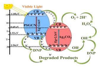
**Fig. 9** Mechanism for enhanced photocatalytic activity of Ag<sub>2</sub>-CO<sub>3</sub>/PSGCN.
