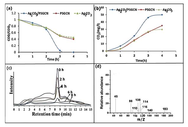
**Fig. 10** (a) COD and (b) CO<sub>2</sub> estimation during mineralization process. (c) HPLC and (d) LCMS analysis during degradation of DNP.  $[DNP] = 1.0 \times 10^{-3} \text{ mol dm}^{-3}$ ; [photocatalyst] = 50 mg/100 mL; initial reaction pH = 4.0 and Light intensity = 750 l×.
