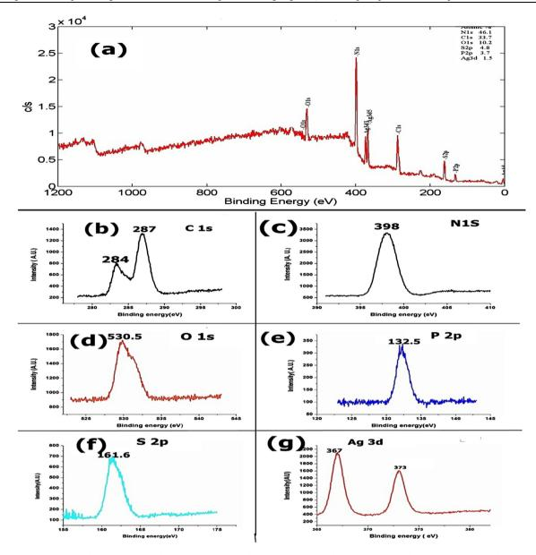
Fig. 5 XPS (a) whole spectrum of  $Ag_2CO_3/PSGCN$ , (b) C1s, (c) N 1s, (d) O1s, (e) P 2p, (f) S2p and (g) Ag 3d spectra.
