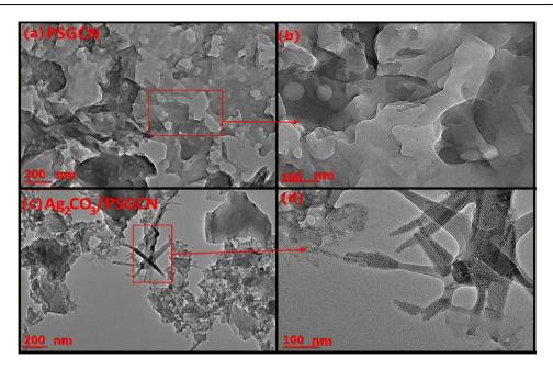
Fig. 2 (a) TEM images of PSGCN, (b) enlarged view of selected area of figure (a), (c) TEM image of  $Ag_2CO_3/PSGCN$  and (d) enlarged view of selected area of figure (c).
