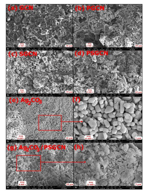
Fig. 1 (a-h). SEM image of (a) GCN, (b) PGCN, (c) SGCN, (d) PSGCN, (e)  $Ag_2CO_3$ , (f) Magnified view of selected area of (e), (g)  $Ag_2CO_3/PSGCN$  and (h) magnified view of selected area of (h).
