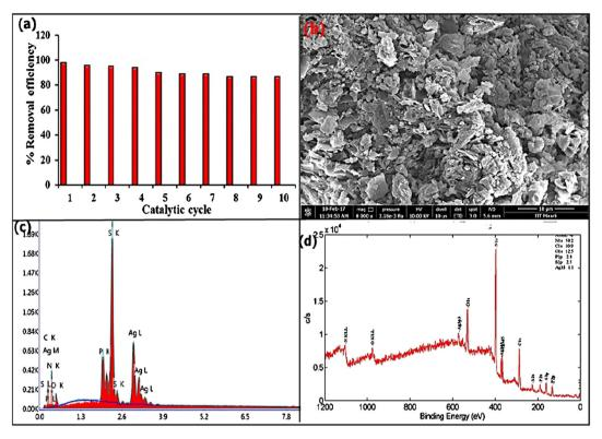
Fig. 11 (a) Recycle efficiency of Ag<sub>2</sub>CO<sub>3</sub>/PSGCN photocatalyst, (b–d) SEM, EDX and XPS image after ten catalytic cycles. DNP] =  $1.0 \times 10^{-3}$  mol dm<sup>-3</sup>; [photocatalyst] = 50 mg/100 mL; initial reaction pH = 4.0 and Light intensity = 750 l×; reaction time = 120 min.
