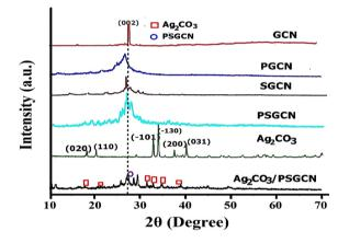
**Fig. 3** XRD analysis of Ag<sub>2</sub>CO<sub>3</sub>/PSGCN, Ag<sub>2</sub>CO<sub>3</sub>, PSGCN, PGCN, SGCN and GCN.
