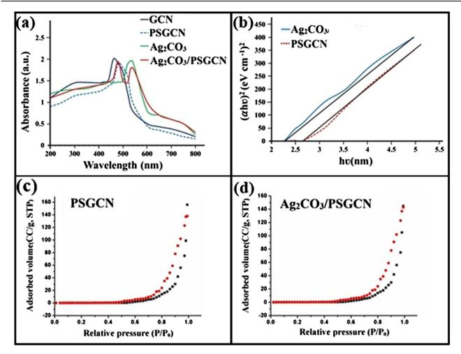
**Fig. 6** (a-d): (a) UV-visible spectrum, (b) Tauc plot of GCN, PSGCN, Ag<sub>2</sub>CO<sub>3</sub> and Ag<sub>2</sub>CO<sub>3</sub>/PSGCN, (c and d) BET isothern of PSGCN and Ag<sub>2</sub>CO<sub>3</sub>/PSGCN.
