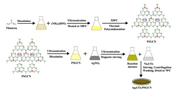
Scheme 1 Preparartion of Ag<sub>2</sub>CO<sub>3</sub>/PSGCN photocatalyst.
