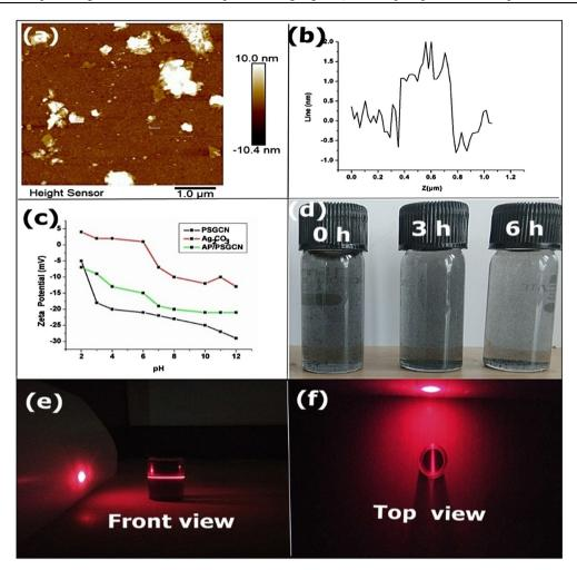
Fig. 7 (a) AFM analysis  $Ag_2CO_3/PSGCN$  (b) Z line profile for  $Ag_2CO_3/PSGCN$ , (c) zeta potential of PSGCN,  $Ag_2CO_3$  and  $Ag_2CO_3/PSGCN$  and (d) dispersion effect and (e and f) Tyndall effect in  $Ag_2CO_3/PSGCN$ .
