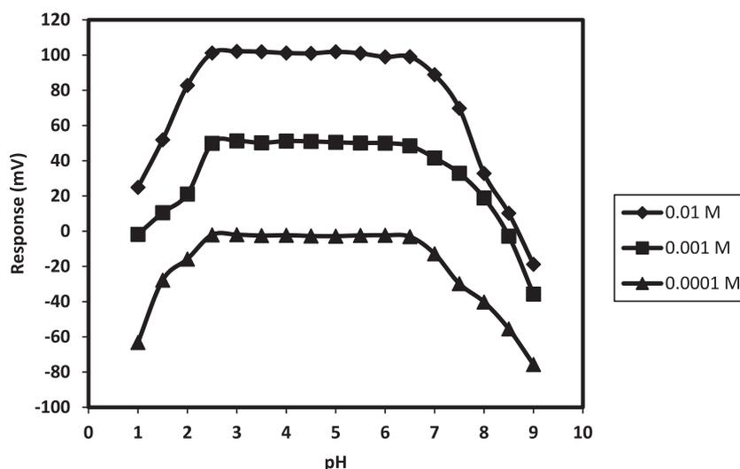
**Figure 5** Effect of pH on the response of proposed sensor No. 1 (pH range 2.5–6.5).
