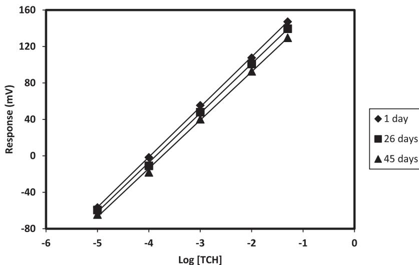
Figure 6 Calibration curve of sensor No. 1 as a function of time.
