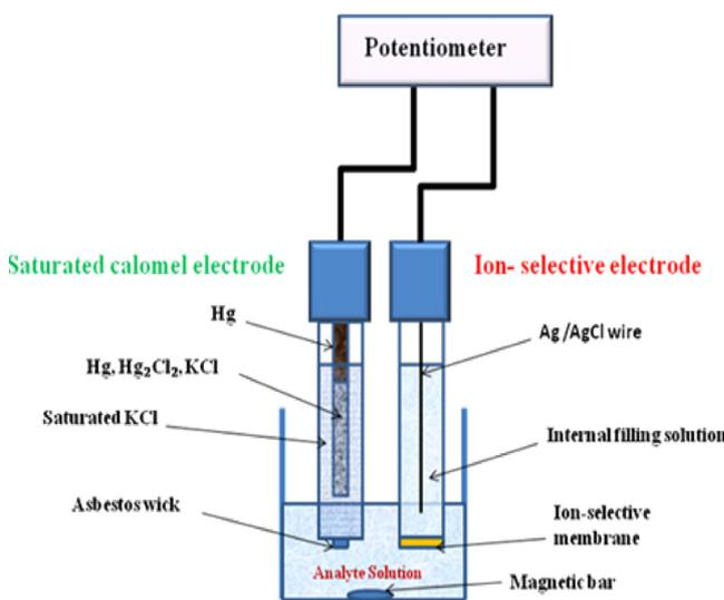
**Figure 2** Schematic diagram of a conventional ion-selective membrane, measuring cell.
