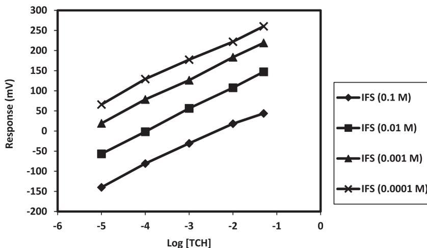
**Figure 4** The effect of the internal filling (IFS) solution on the response of the tetracaine – selective electrode using sensor No. 1 based on (TC-PTA) ion-pair complex with DBPH as a plasticizer.
