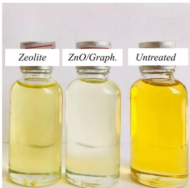
**Fig. 8** The visual aspect of the oil-treated by ZnO/Graphene composite, aged oil and the oil treated by the commercial zeolite.
