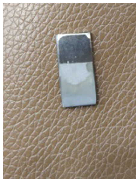
Fig. 5 Shows an optical photograph of a sample of Ti both unpolished and polished regions in 1 ChCl: 2 PG.
