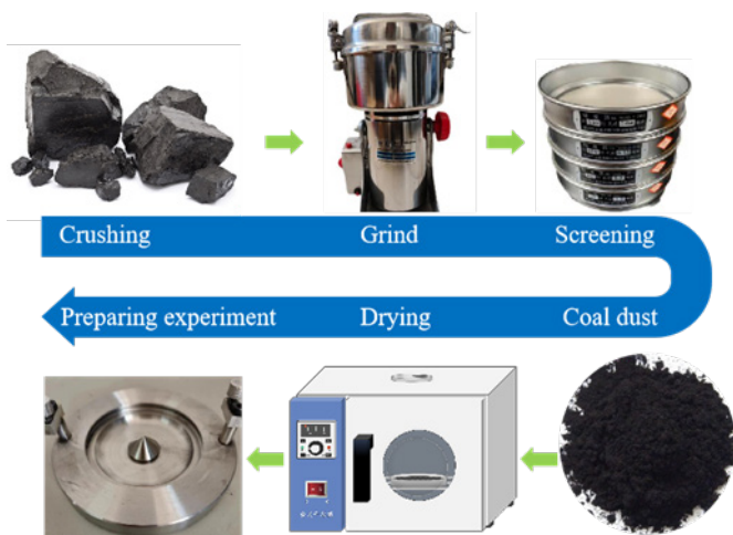
Figure 4. The experimental procedures include crushing, grind, screening, getting coal dust, drying, and preparing for the experiment. Source: Drawn by Zemiao Yang.
