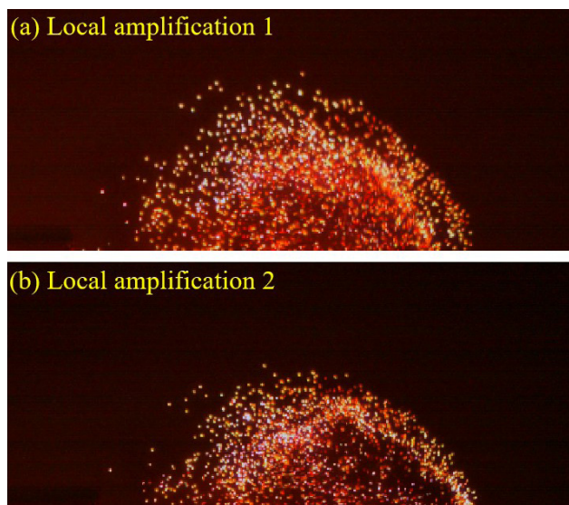
Figure 12. Coal dust flame propagation edge. (a) Local amplification 1 (b) Local amplification 2.
