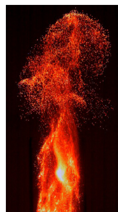
Figure 11. Coal dust flame propagation under high-speed camera.
