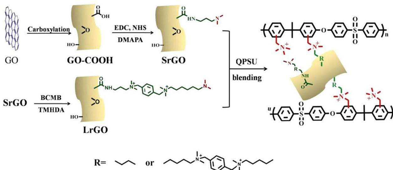
**Fig. 16** The chemical synthesis of functionalized rGO and their crosslinked QPSU-based AEMs. Copyright permission was obtained from Elsevier 2019 for the redrawn figure (Bai et al., 2019).
