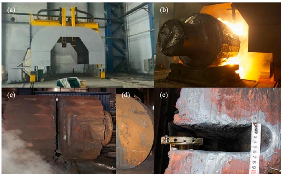
Fig. 24. Flame cutting test of ultra-large section steel ingot.
