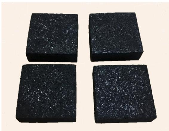
Fig. 1. Some examples of fully cured SG/CHH -filled poly(BA-35x) composite samples.
