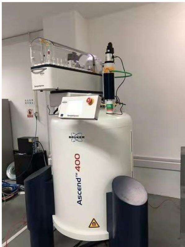
**Fig. 2** Brooke 400 M solid-state nuclear magnetic resonance instrument.
