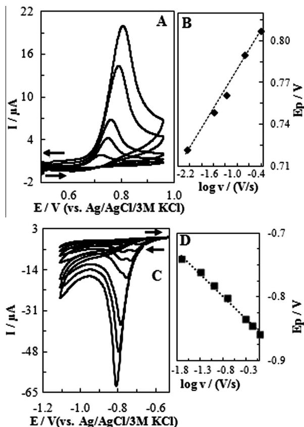
**Figure 3** CVs of CTP solutions with different scan rates in 0.04 M BR on (A) GC (scan rates from lower to higher; 0.01, 0.05, 0.30, 0.75 V/s, pH 4.0,  $C_{CTP} = 0.85$  mM), (B) dependency of peak potential to logarithm of scan rate, (C) HMDE (scan rates from lower to higher; 0.02, 0.05, 0.10, 0.30, 0.50, 0.70, 1.00 V/s, pH 6.0,  $C_{CTP} = 0.75$  mM), and (D) dependency of peak potential to logarithm of scan rate.
