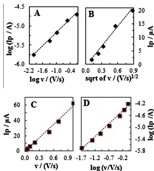
**Figure 4** (A) dependency of logarithm of peak current to logarithm of scan rate on GCE, (B) dependency of peak current to square-root of scan rate on GCE, (C) dependency of peak current to scan rate on HMDE, and (D) dependency of logarithm of peak current to logarithm of scan rate on HMDE.
