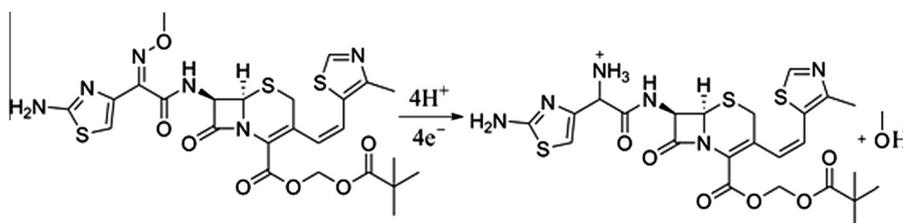
**Scheme 2** One of the possible reduction mechanisms for CTP on HMDE.
