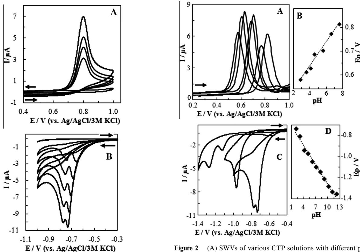
**Figure 1** CVs of various CTP solutions in 0.04 M BR with scan rate of 0.10 V/s, on (A) GC (concentrations from lower to higher; blank, 0.25, 0.45, 0.65, 0.85 mM; pH 4.0) (B) HMDE concentrations from lower to higher; blank, 0.10, 0.25, 0.48, 0.75, 1.00 mM; pH 6.0.
