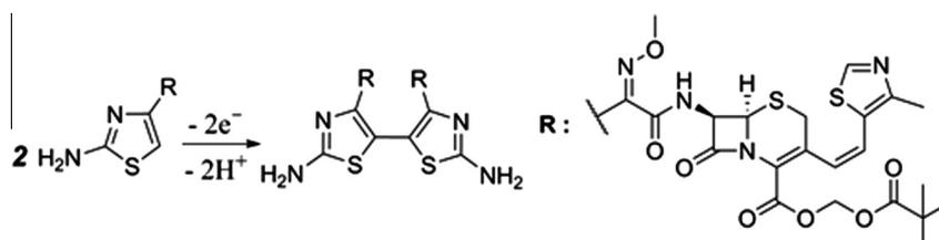
**Scheme 1** Proposed oxidation mechanism of CTP on GCE.
