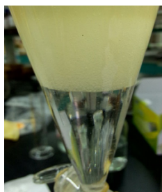
Fig. 4 The mixture after adding saturated sodium chloride.
