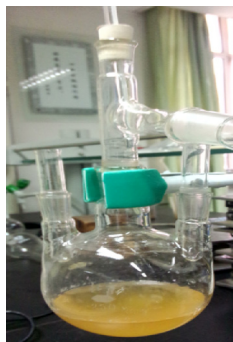
Fig. 5 The citric acid isopentyl ester obtained after distillation.
