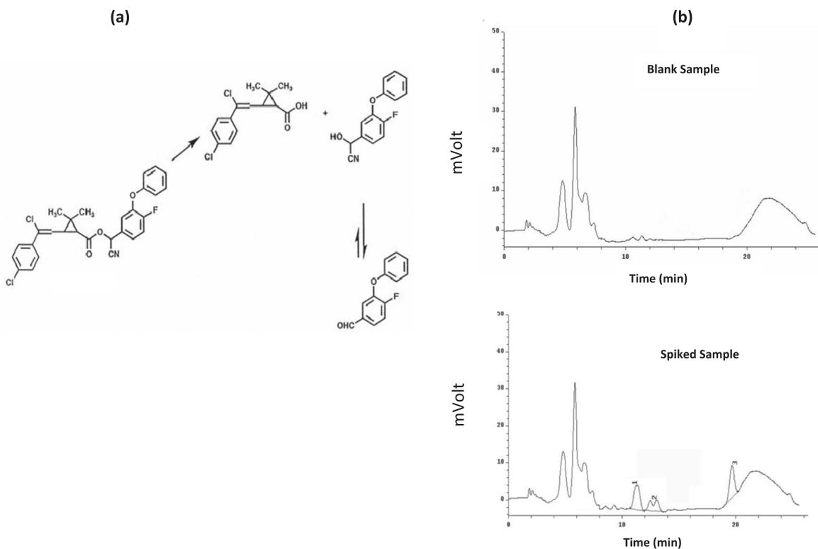
**Fig. 6** (a) Photo irradiated obtained fluorescent active product of flumethrin; (b) A SPME-HPLC-PIF-FD chromatogram retrieved by analysis of Jajroud river water samples an blank sample and spiked sample with (1) cyfluthrin, (2) cypermethrin, and (3) flumethrin. pyrethroids at 10  $\mu\text{g/L}$  under optimized conditions. Reprinted from (Bagheri et al., 2009) with the permission from Wiley.
