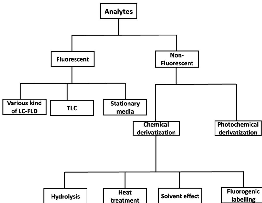
Fig. 1 Schematic view of the various fluorescence approach for analysis of analytes.
