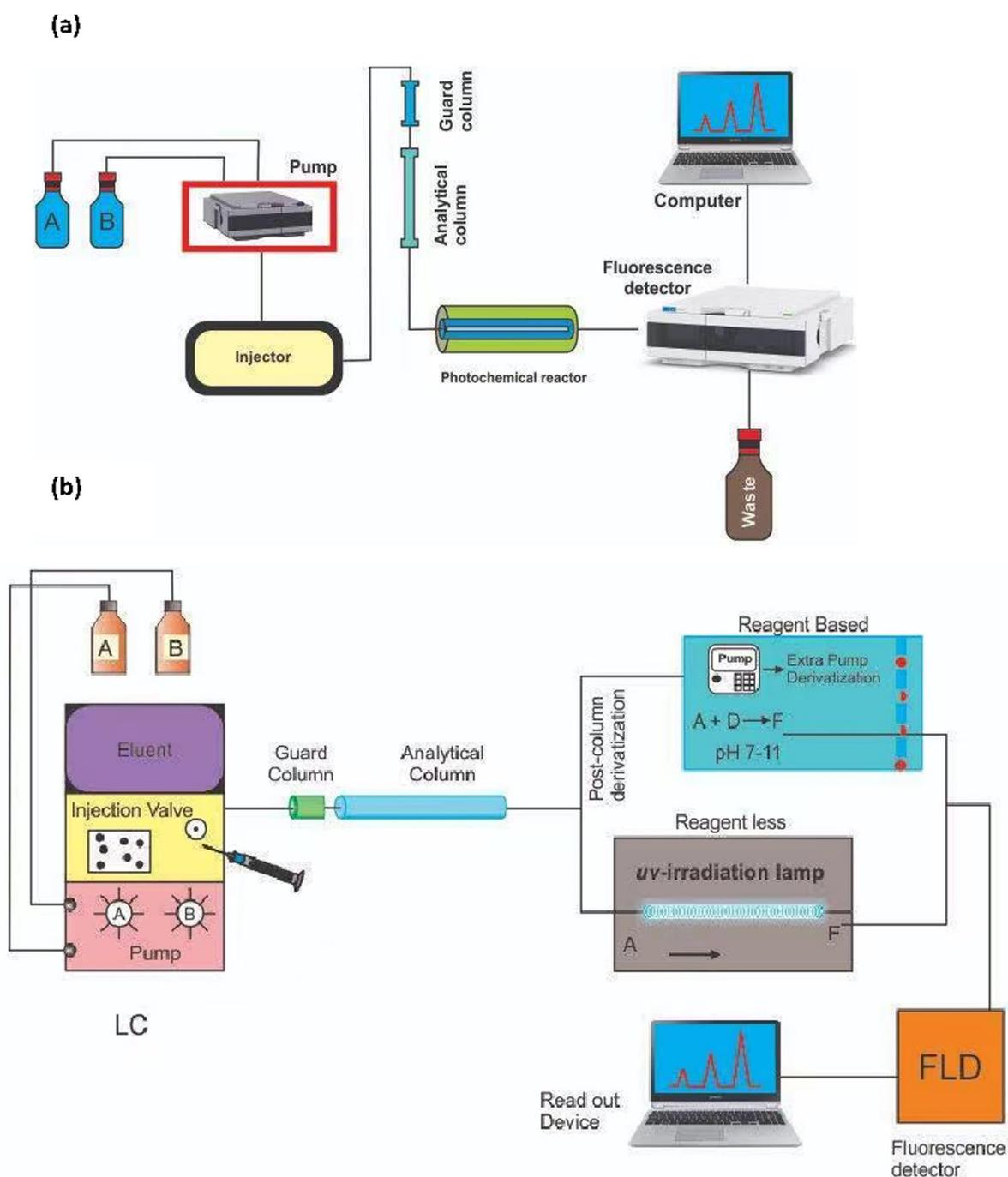
**Fig. 2** Systematic diagram of (a) liquid chromatography coupled with post-column UV irradiation fluorescence detection system; (b) comparison of post-column reagent-based and UV irradiation-based derivatization.
