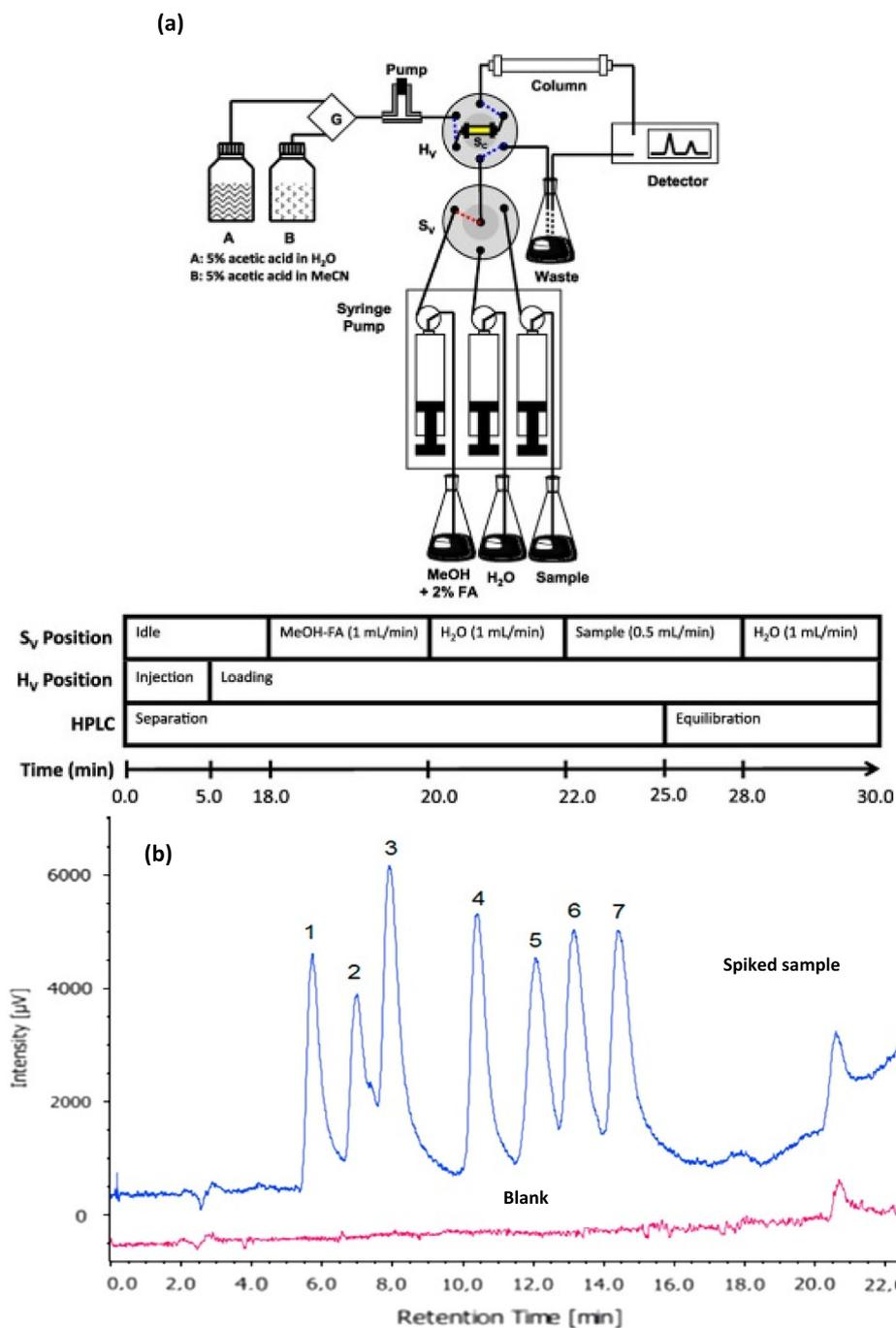
**Fig. 4** (a) On-line SPE-LC-PIF-FLD setup; (b) On-line SPE-LC-PIF chromatogram of a blank and human serum sample spiked with seven sulfonamides at 30 mg/L, whereas i: sulfadiazine, ii: sulfapiridine, iii: sulfamerazine, iv: sulfa-methazine, v: sulfachloropiridazine, vi: sulfamethoxazole, vii: sulfadoxine. Reprinted from Arroyo-Manzanares et al., 2015 with the permission from Elsevier.
