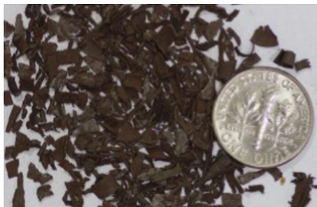
Figure 1  $\text{Fe}^0$  aggregate catalyst.
