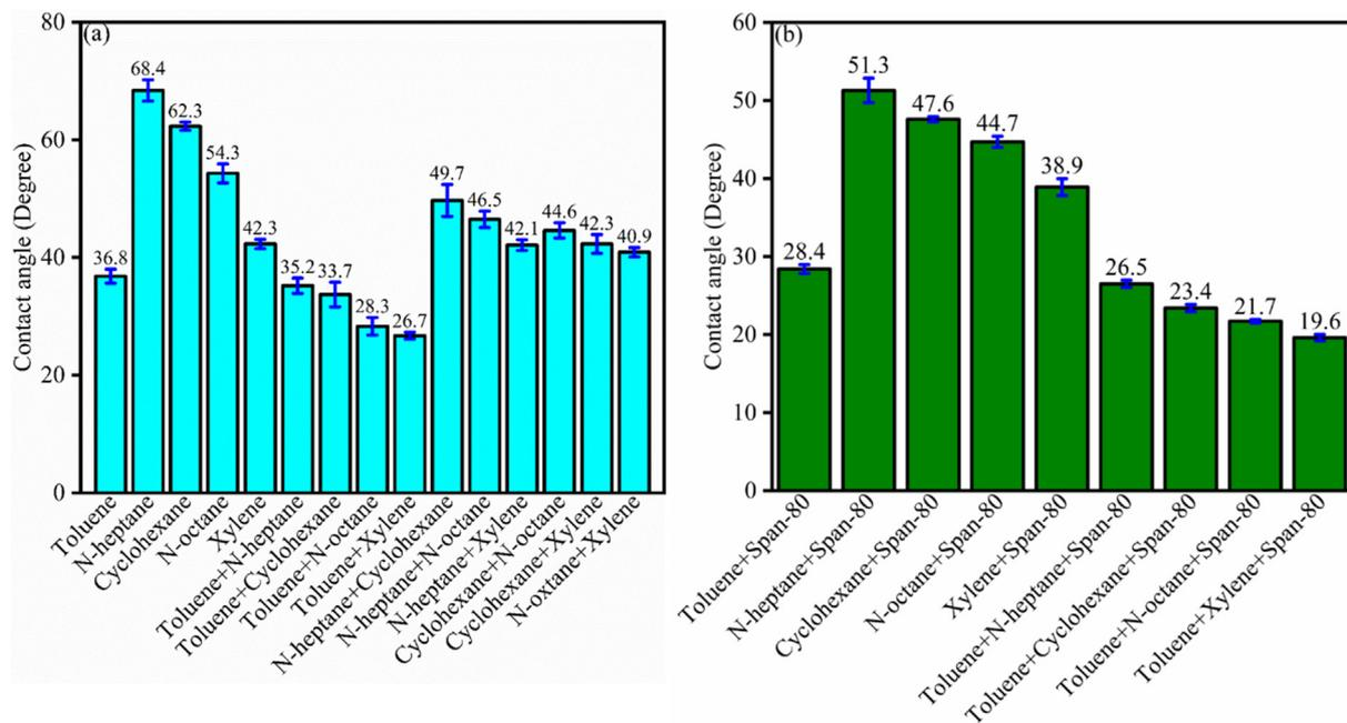
Fig. 4 The contact angle of the sands extracted by (a) Single/complex solvents; (b) Span 80 enhanced single/complex solvents.
