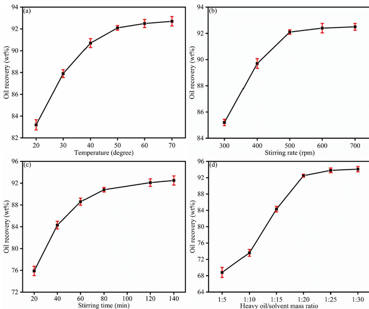
**Fig. 1** The (a) temperature ( $^{\circ}\text{C}$ ); (b) stirring rate (rpm); (c) stirring time (min); (d) heavy oil/solvent mass ratio effect on oil recovery (wt %).
