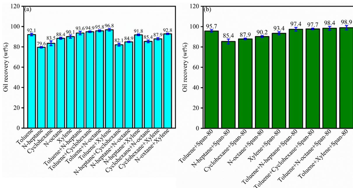
**Fig. 2** (a) Single/complex solvents; (b) Span 80 enhanced single/complex solvents extraction for oil recovery.
