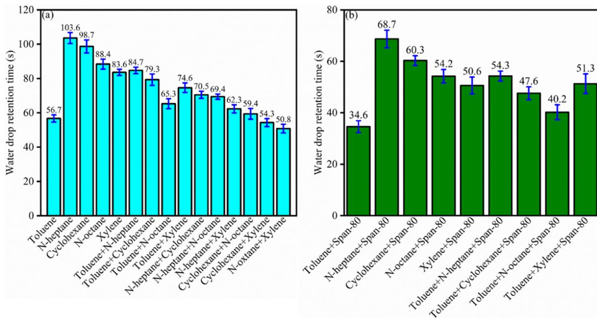
Fig. 5 The water drop retention time (s) of the sands extracted by (a) single/complex solvents; (b) Span 80 enhanced single/complex solvents.
