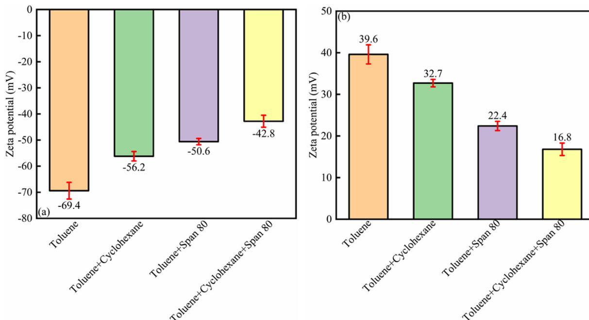
Fig. 9 The zeta potentials of (a) heavy oil; (b) sands extracted by different methods in deionized water.
