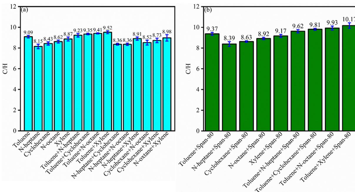
Fig. 3 The C/H ratio of heavy oil extracted by (a) Single/complex solvents; (b) Span 80 enhanced single/complex solvents.
