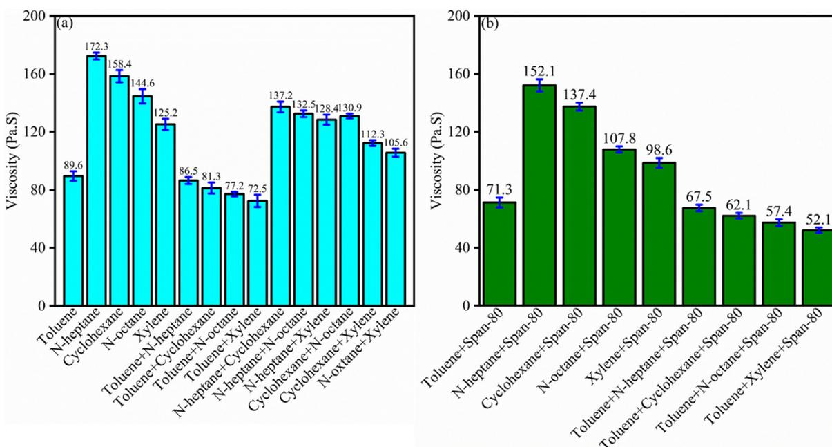
Fig. 6 The viscosity of heavy oil extracted by (a) Single/complex solvents; (b) Span 80 enhanced single/complex solvents.
