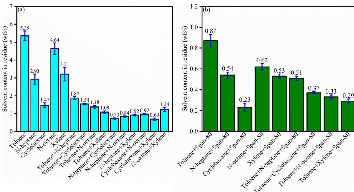
Fig. 7 (a) Single/complex solvents; (b) Span 80 enhanced single/complex solvents residue content in sands.
