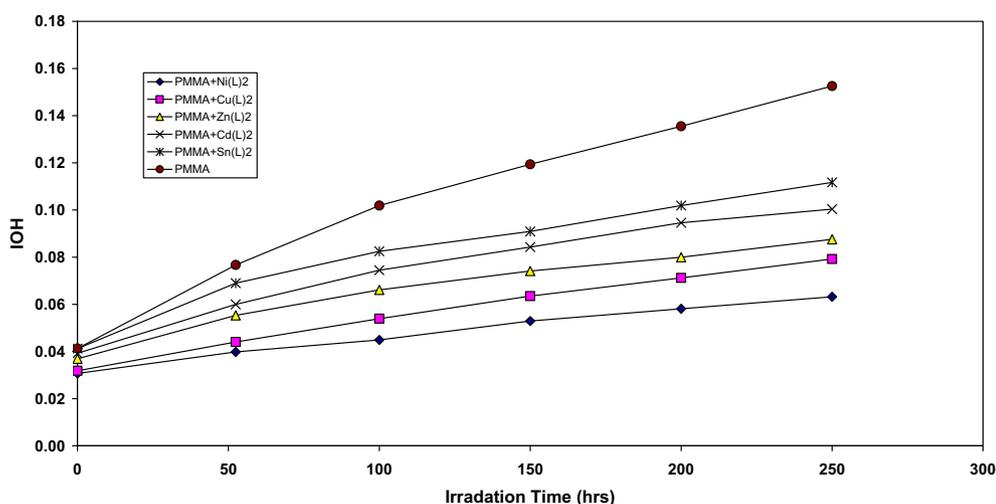
**Figure 1** The relationship between the hydroxyl index and irradiation time for PMMA films (40  $\mu\text{m}$  thickness). Containing different additives, concentration of additives are fixed at 0.5% by weight.
