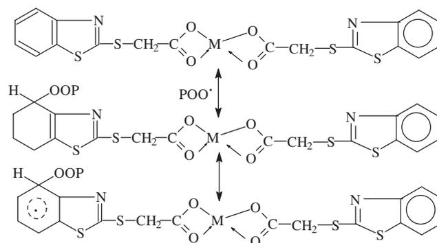
**Scheme 2** Suggested mechanism of photostabilization of carboxylates complexes as radical scavengers through energy transfer and forming un-reactive charge transfer and stabilize through resonating structure.
