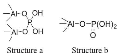
**Scheme 1** The structure of Phosphoric acid supported on alumina.
