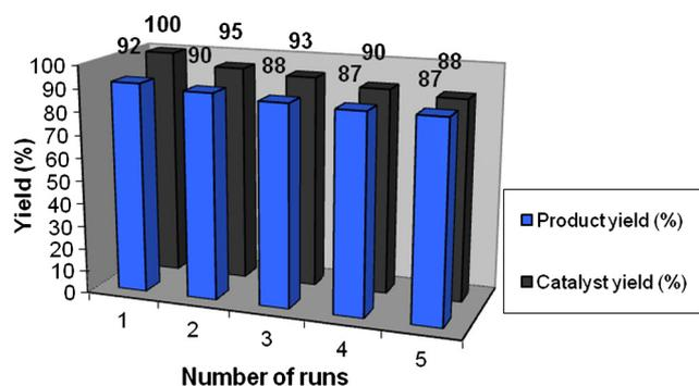
**Figure 1** The investigation of the recycling of  $\text{H}_3\text{PO}_4/\text{Al}_2\text{O}_3$ .
