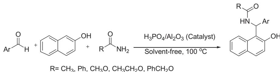
**Scheme 2** Synthesis of  $\alpha$ -amidoalkyl- $\beta$ -naphthols and  $\alpha$ -carbamato-alkyl- $\beta$ -naphthols.
