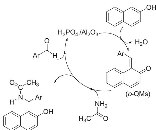
**Scheme 4** The suggested mechanism for preparation of  $\alpha$ -amidoalkyl- $\beta$ -naphthol derivatives.
