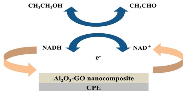
**Scheme 1** Schematic representation for the bioelectrocatalytic sensing of ethanol through the catalytic oxidation of NADH using  $\text{Al}_2\text{O}_3$ -GO nanocomposite modified CPE electrode.
