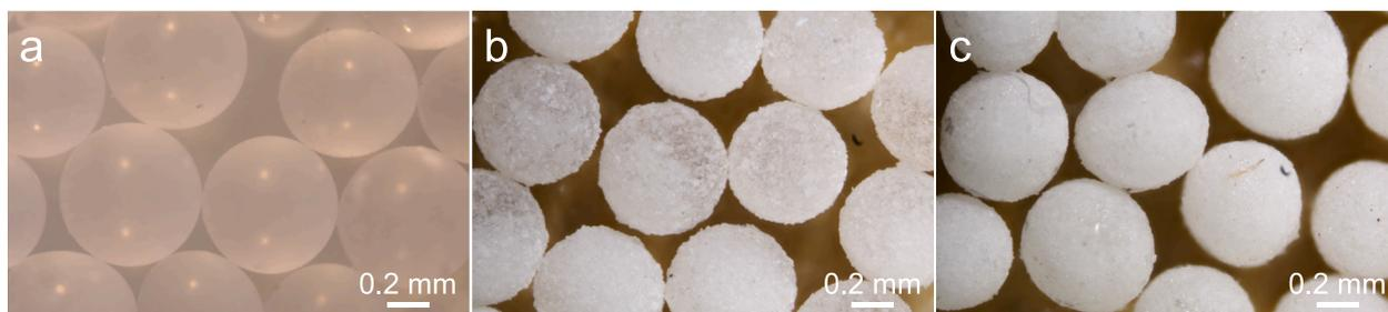
Fig. 2. Optical images of (a) poly(MMA-co-St), (b) poly(MMA-co-St)/20 wt% Dia, and (c) poly(MMA-co-St)/40 wt% Dia.
