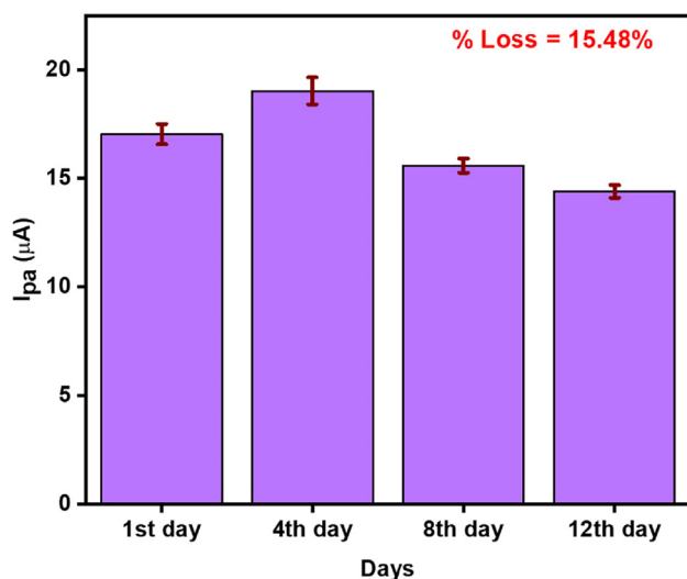
Fig. 12 Inter-day stability studies of CNC/CuTMePP/GC in 0.50 mM DA (0.1 M phosphate buffer, pH = 7) using DPV.
