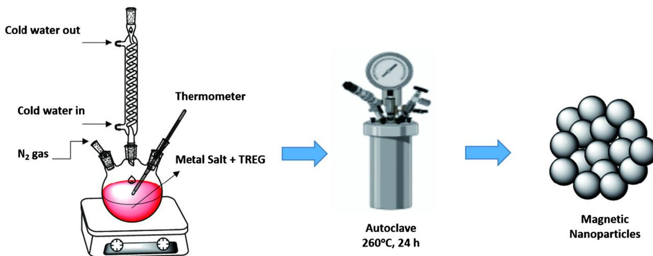
Fig. 3 The synthesis of  $\text{Fe}_3\text{O}_4$  and monodisperse  $\text{CuFe}_2\text{O}_4$  through solvothermal method by Fotukian et al. (2020).
