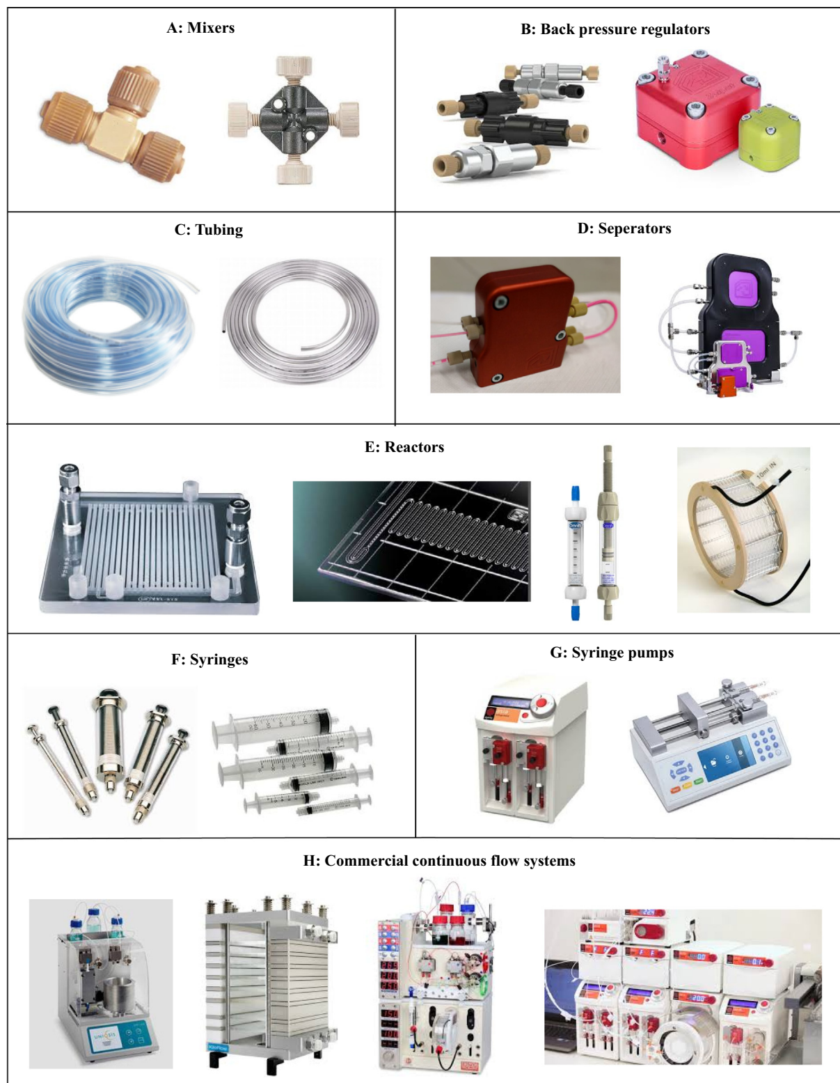
Fig. 2 Typical continuous flow components and systems.
