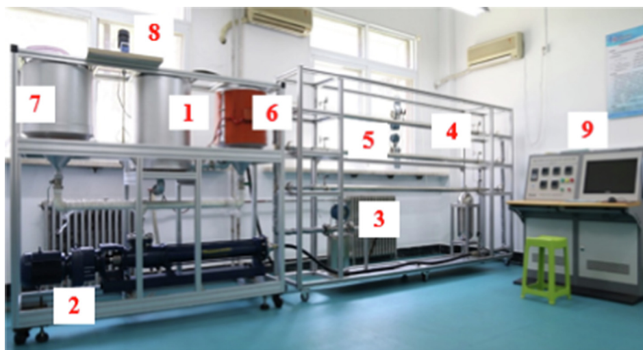
Fig. 2 Friction reduction rate pipeline test system for polymer fluid.
