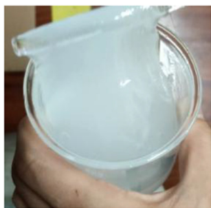
Fig. 24 Hanging state of 0.10 wt% CND + 0.60 wt% FR-900.
