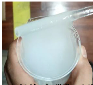
Fig. 23 Hanging state of 0.05 wt% CND + 0.60 wt% FR-900.
