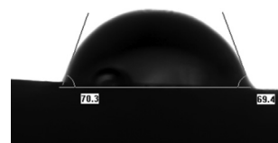
Fig. 12 Contact angle of oil droplets on core surface before wetting and modification, “water-oil-solid” Average contact angle = 69.9°.
