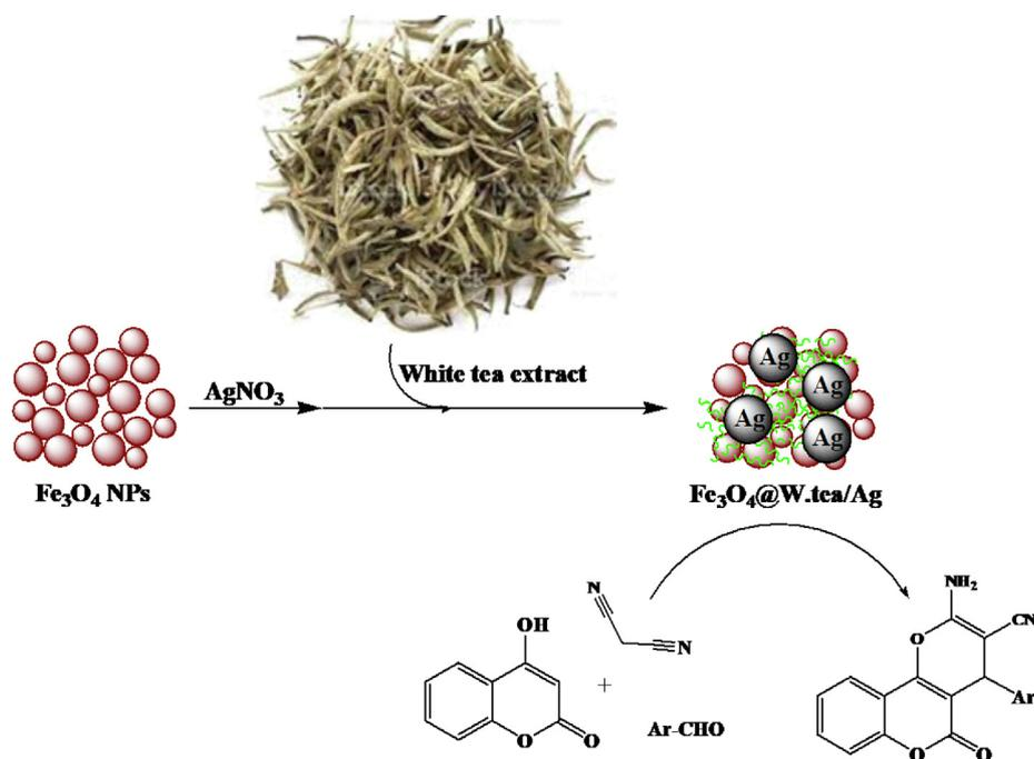
**Scheme 1** Schematic green synthesis of Fe<sub>3</sub>O<sub>4</sub>@W.tea/Ag nanocomposite mediated by *White tea* extract and its applications for synthesis of pyrano[3,2-*c*]chromene derivatives.
