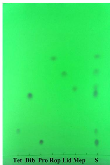
**Fig. 1** TLC plates under 254 nm UV light irradiation for separation of six anesthetics with  $R_f$  values of 0.09 (Pro), 0.17 (Tet), 0.41 (Dib), 0.50 (Mep), 0.62 (Lid) and 0.73 (Rop), respectively. Developing system: cyclohexane-triethylamine system (7:3). The concentrations were 2 mg mL<sup>-1</sup> for Pro, Tet, Dib, and 5 mg mL<sup>-1</sup> for Mep, Lid, Rop, respectively.
