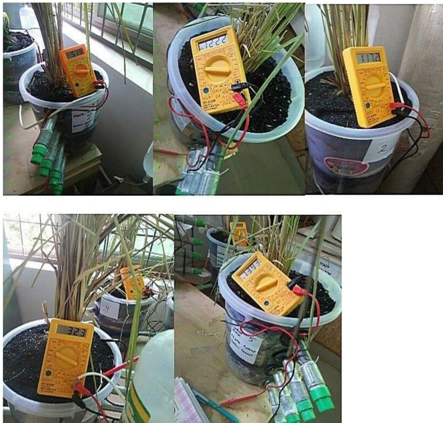
**Fig. 10** Maximum average voltage output of five different configurations of CW-MFCs.
