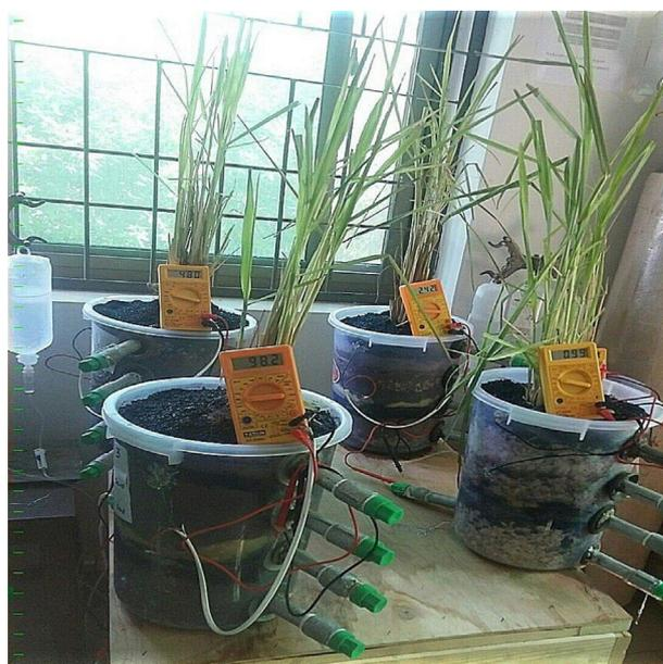
**Fig. 2** Photograph of five reactors with different configurations of Constructed wetlands microbial fuel cells (CW-MFCs) designed by *Cymbopogon nardus*.
