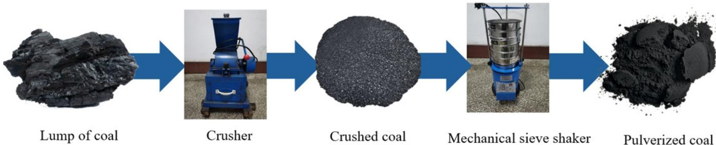
Figure 1. Coal sample preparation process.
