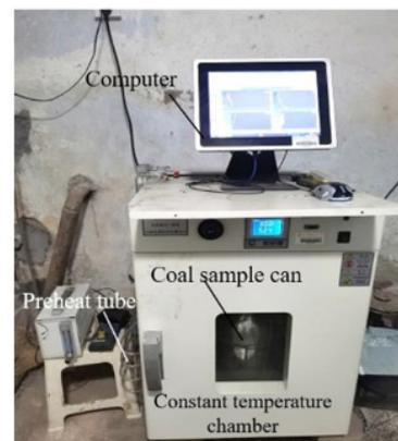
Figure 2. Sealed oxidation experimental apparatus.
